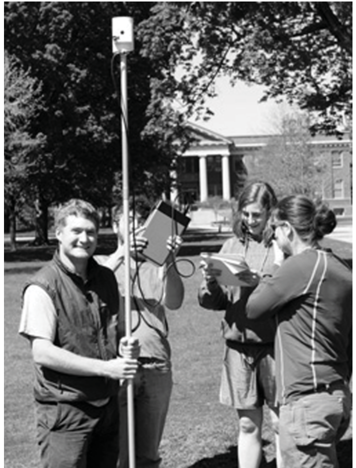
Students in geophysics use a magnetometer to survey the Bald spot.
