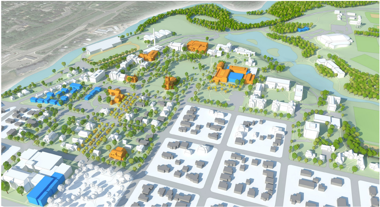
/ Figure 4 / Recommended campus plan showing renovated existing campus buildings, in orange, and new construction, in blue
