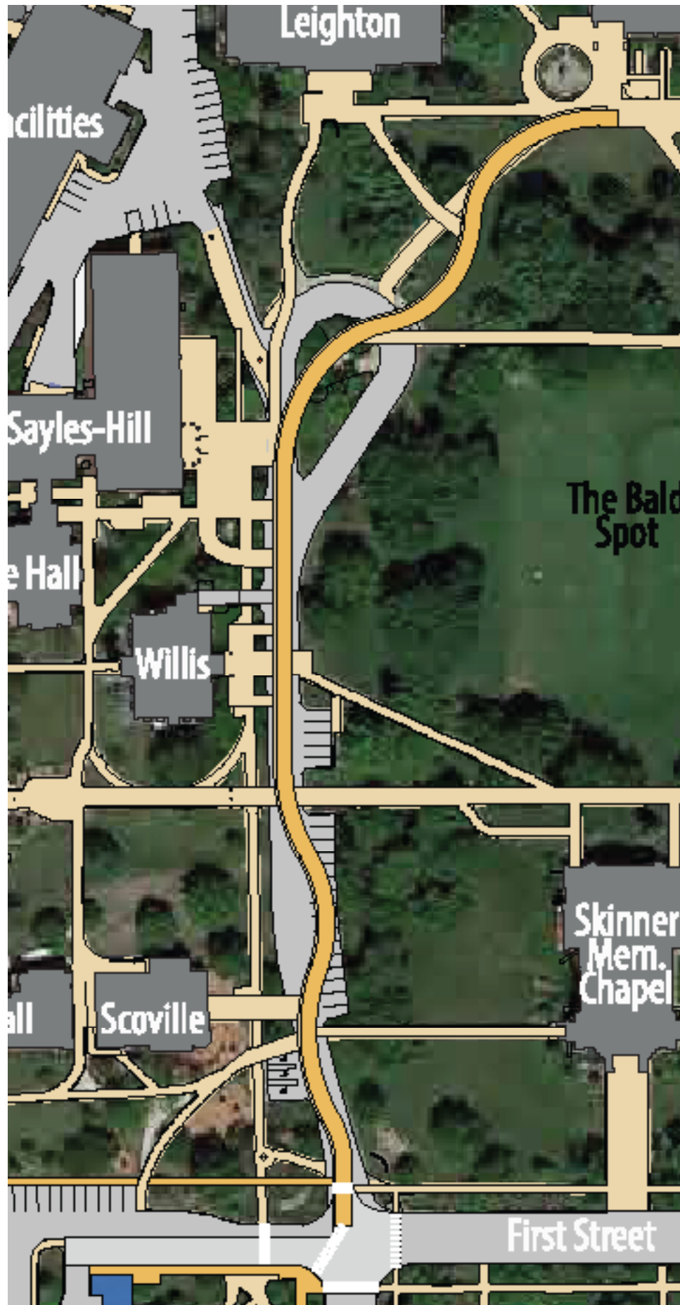
5.b College Street Alternate: 12' sidewalk for pedestrians, bikes, and emergency traffic only
